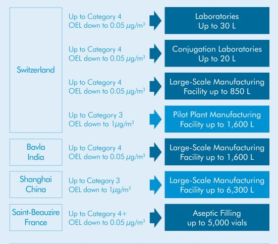
NB: Containment is ensured through rigid barrier isolation systems and flexible segregation of key equipment. Results are validated by containment testing performed according to ISPE's SMEPAC-guideline. \* Result of surrogate containment testing: 0.01 µg/m<sup>3</sup>
